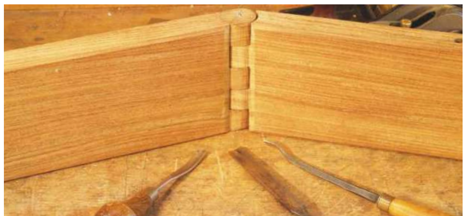
▲ Pic.15 The completed joint, showing the gouges used
